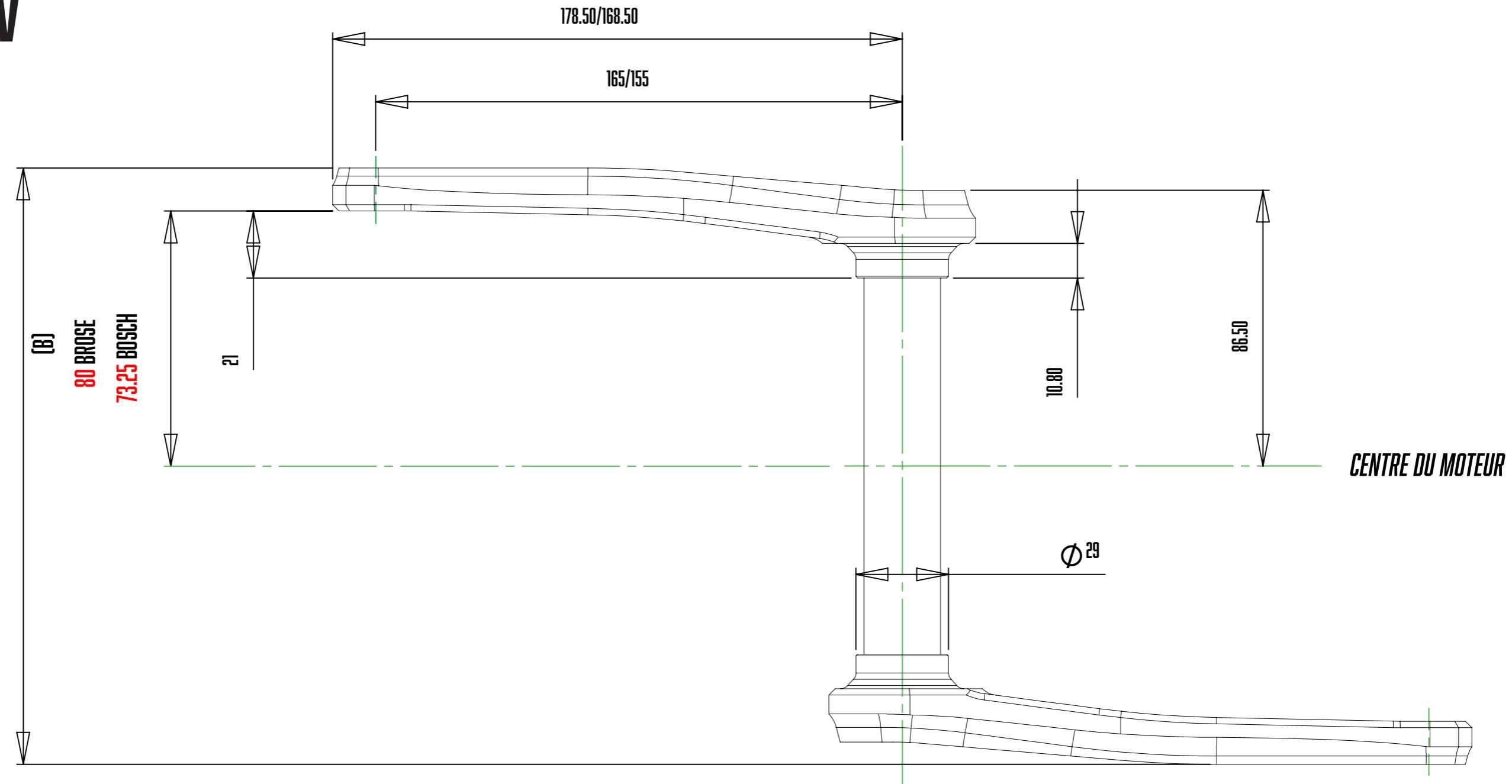
\*CE MODÈLE DE MANIVELLES EST PLUS ADAPTÉ AUX MOTORISATIONS BROSE, PEUT ÉGALEMENT CONVENIR AUX MOTORISATIONS BOSCH (GEN 2/4) SI LE DÉGAGEMENT DES BASES DE CADRE EST SUFFISANT (Q-FACTOR ÉTROIT). (NON COMPATIBLE AVEC LES MOTORISATIONS BOSCH DE GÉNÉRATION 3)
