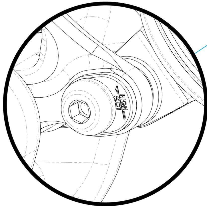
The laser etched flip chip should be located on the drive side. The arrow pointing up indicates in which setting the geometry is. For instance, on picture beside "LOW" setting. Turn both flip chip 180° to change the geometry setting.
